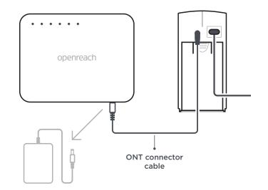
The ONT **Power** light should be on or flashing to indicate it is working. The battery takes 24 hours to become fully charged and the ONT can still be used in the meantime.
