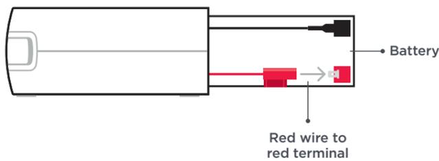
Then slide the battery in fully and replace the cover.
