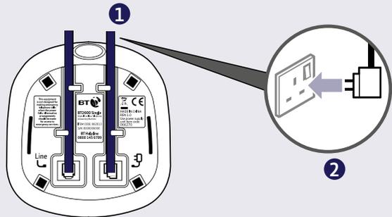
The phone line cord is pre-installed but **don't** plug the other end into the wall socket yet.
