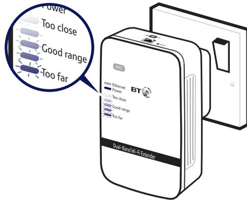
☰ If the range lights continue to scroll add up and down for more than 1 minute. Check your hub/router is switched on and try moving your extender closer to it.
