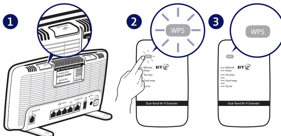
**Note:** the WPS button is only used to connect to the router and can't be used to connect devices.
