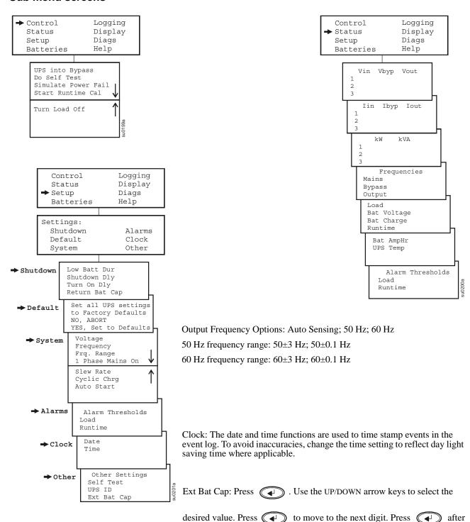
selecting the final value, to lock in the battery capacity setting.
