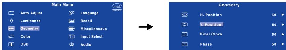
An adjustment page appears after you press the ENTER Button. Then, use the ◀ / ▶ Buttons to change the vertical position settings. The vertical position of the overall display should be changing accordingly while you are doing this.
