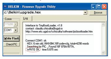
7. Disconnect the Serial Flash Cable, **POWER OFF** the KVM Switch, set the DIP switch back to the Normal Run Operation position "ON, ON", and then power on the KVM Switch. The KVM Switch should be running on the new firmware. The OSD will display the FW version in the bottom-right corner of the "Main Menu" page.
