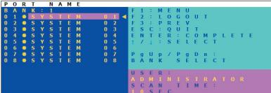
The main OSD menu displays the current selected BANK and connected servers to that BANK. If you have only one PRO3 KVM Switch in your configuration, the OSD menu will display "BANK 00". A "☒" symbol indicates that the connected server is powered up.
