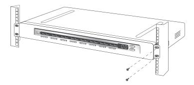
**Note:** If this PRO3 KVM Switch will be daisy-chained to another KVM switch, set the BANK address prior to installing on a rack. Refer to the section in this User Manual titled "Connecting Multiple PRO3 KVM Switches (Daisy-Chaining)".
