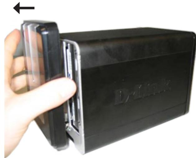
3. Insert a 3.5" SATA hard drive into each available drive bay. Make sure to align the drive connectors to the SATA connectors on the bottom edge inside the drive bay of the DNS-323. Gently push the drive in until it connects. When a drive is inserted properly, you will feel it "seat" into the connector. Some hard drives that are thin or oddly shaped may need to be guided carefully into position. If a drive is not properly seated, the light will not illuminate after powering on the device.
