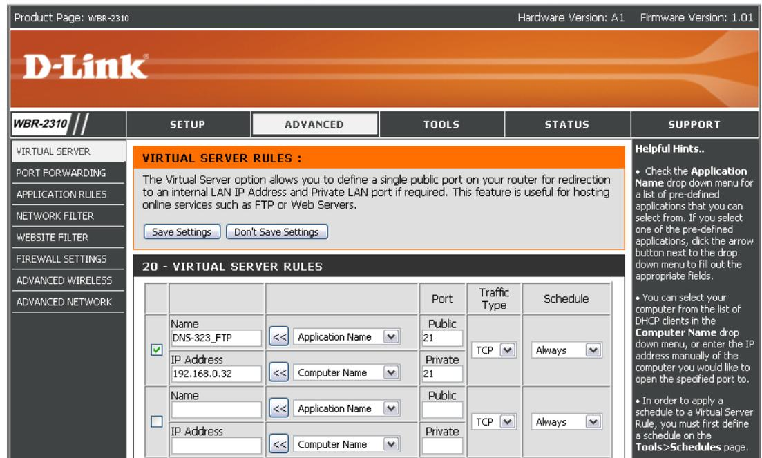
If you use an FTP port other than 21, then users accessing the FTP server using an FTP client will have to specify the non-standard port, and users who are using a browser will have to specify the port in the URL (e.g. ftp://ftp.dns323.com:3000, where the FTP port is 3000).
