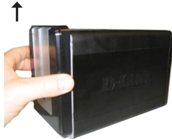
2. Once the faceplate is unlatched, pull it off the device, exposing the drive bays.
