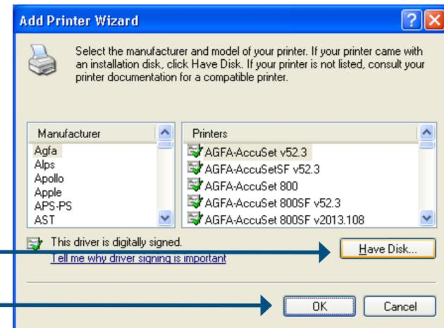
Select the appropriate printer driver from the list and click **OK** to complete the wizard. If the driver is not in the list, select **Have Disk**.
