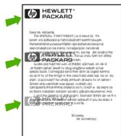
This type of defect might occur when using preprinted forms or a large quantity of narrow media.
