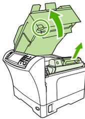
2. Grasp the print cartridge by the handle, and remove it from the device.
