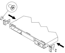
Secure clip-nuts to the rack, and attach brackets with provided screws.
