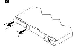
Two-post rack-mounting: Utilize the bracket holes that are offset 6.25".
